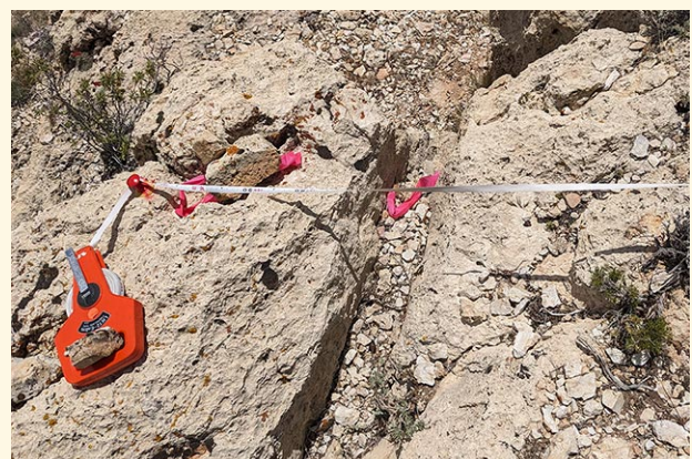
Figure 7 (above). Each of the eight plots (with one exception) was a line across a ledge anchored at a beginning with a 6 in carriage bolt glued into the rock and etched with the plot ID on the top. Figure 8 (below). An end bolt and 30 m tape.
