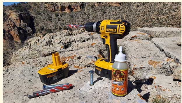
Figure 7 (above). Each of the eight plots (with one exception) was a line across a ledge anchored at a beginning with a 6 in carriage bolt glued into the rock and etched with the plot ID on the top. Figure 8 (below). An end bolt and 30 m tape.
